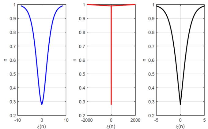
**Fig. 9:**  $n$  is plotted vs.  $\xi$  in weakly relativistic plasma with variation of ion temperature ratio  $\sigma$ . The blue curve denotes  $\sigma = 0.1$ , red denotes  $\sigma = 0.2$ , black denotes  $\sigma = 0.3$ ; other parameters are  $M=0.6$ ,  $F=2/3$  and  $H=2$ .
