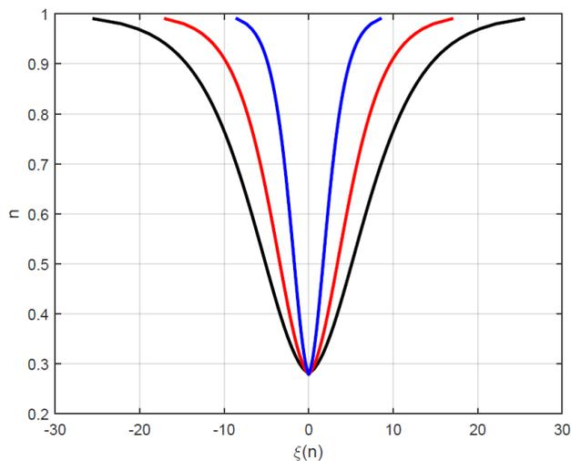
**Fig. 8:**  $n$  is plotted vs.  $\xi$  in weakly relativistic plasma with variation of quantum diffraction parameter  $H$ . The blue curve denotes  $H=2$ , red denotes  $H=4$ , black denotes  $H=6$ . Other parameters are  $M=0.6$ ,  $F=2/3$  and  $\sigma=0.1$ .
